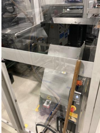
Plastic sprue grinder and dispenser – Injection Molding – Preh Portugal
