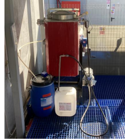
Distillery for solvent waste – Paint Shop – Preh Romania
